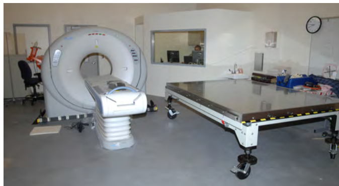
WSU's recently installed 16-slice CT scanner can image certain areas of a horse in just several minutes.
