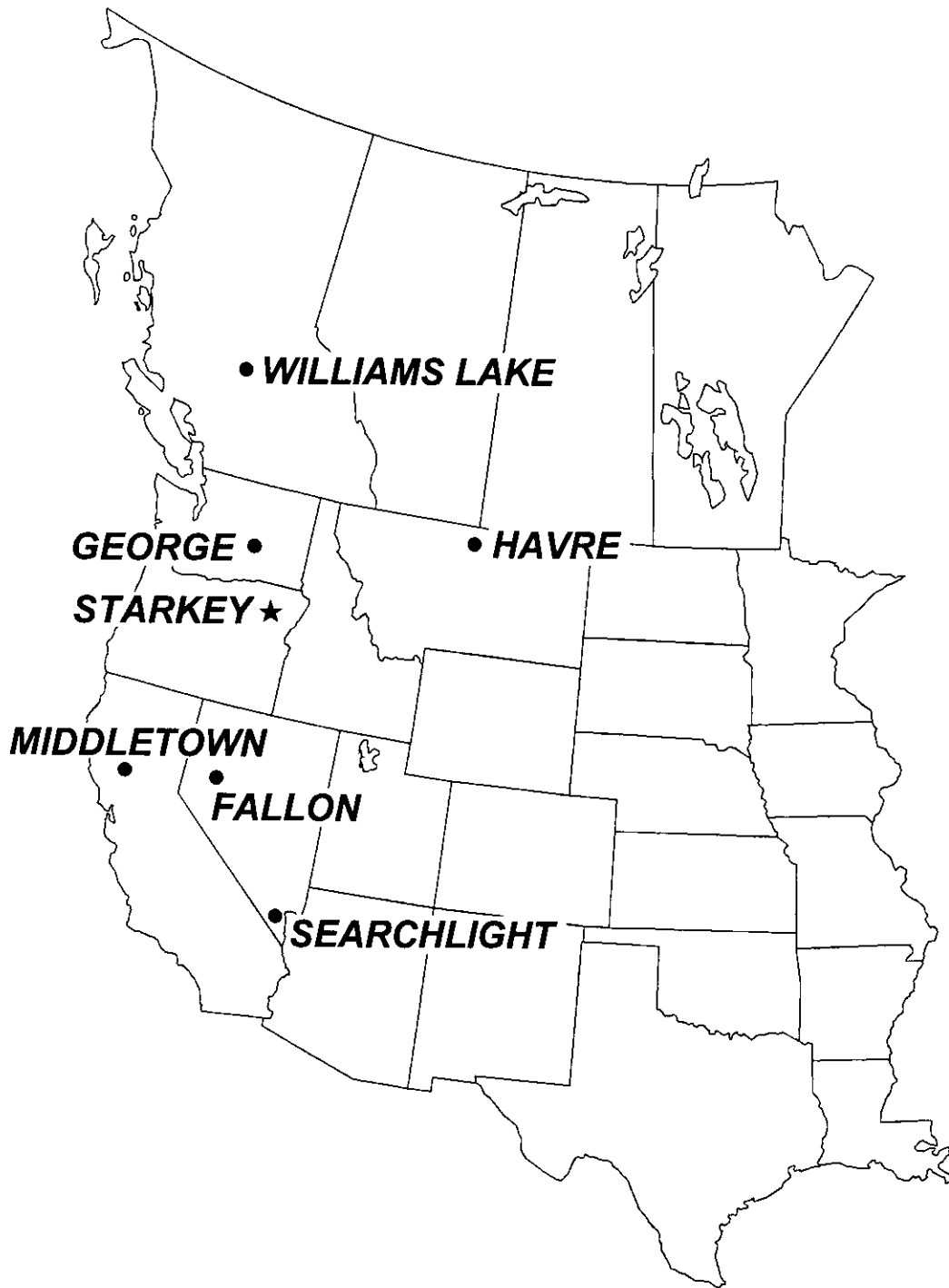
Figure 1. Locations of LORAN-C transmitting towers in the western United States and Canada used to obtain position estimates on the Starkey Experimental Forest and Range, northeast Oregon. LORAN-C transmitting towers at Fallon (Nevada), Middletown (California) and George (Washington) were used in the original automated animal tracking system. These transmitting towers in configuration with those at Williams Lake (British Columbia), Havre (Montana), and Searchlight (Nevada) were used in the upgraded automated animal tracking system.
